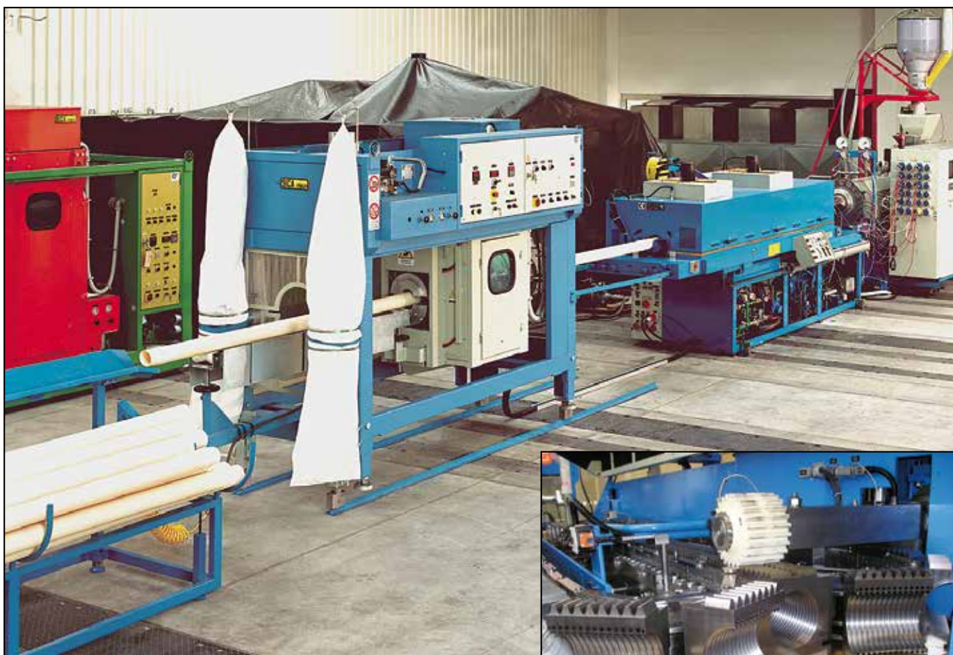
Production of PVC twin wall pipes
