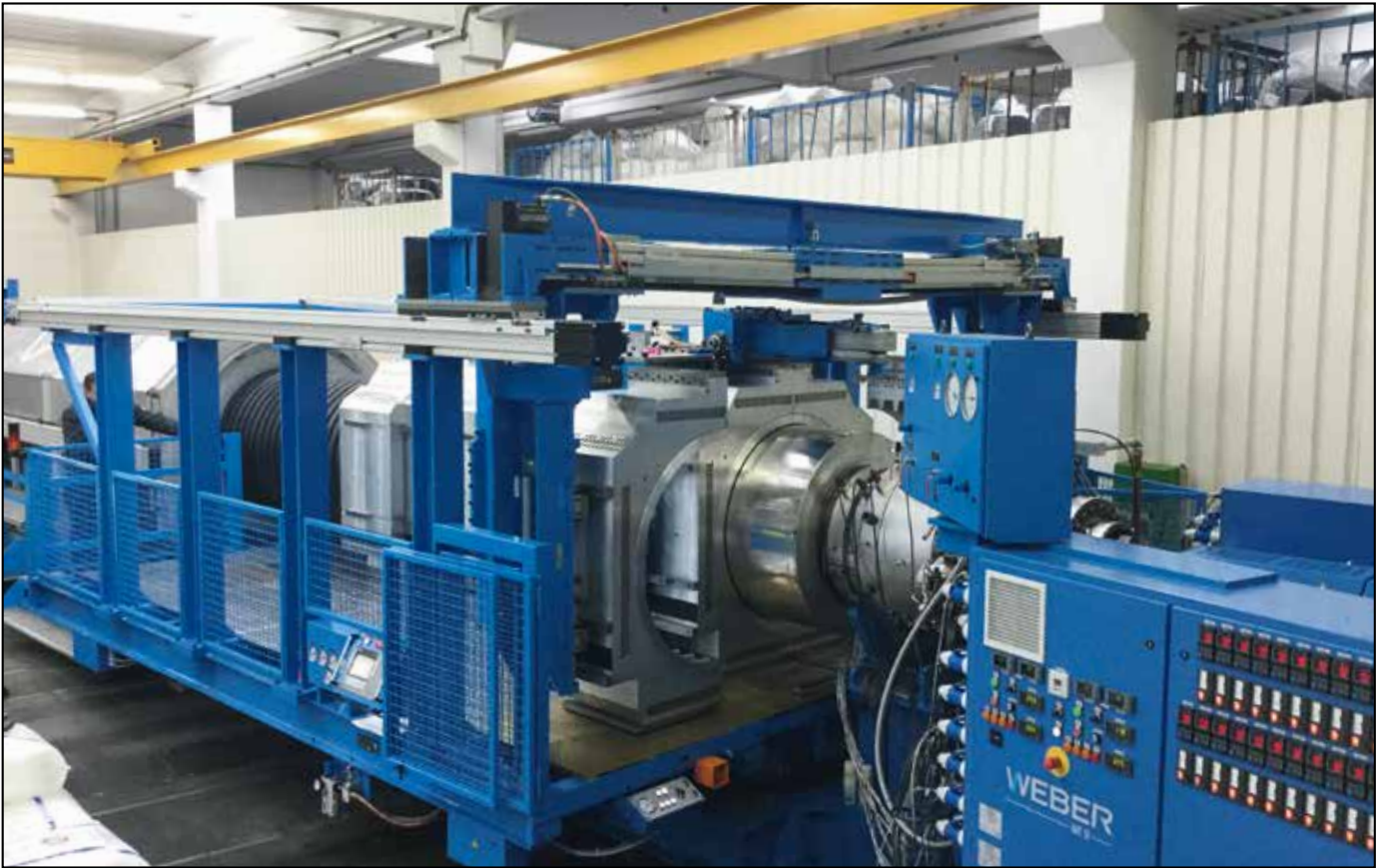
Production of twin wall storm sewer pipes with double-layer integral socket Fig. above: HP 1200 with one conveying bridge; Fig. below: HP 700 with two conveying bridges
