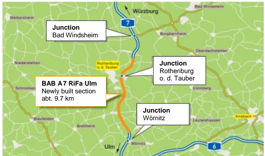
Newly built section of motorway BAB A 7 between junction Bad Windsheim and junction Wörnitz
